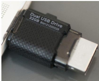
In this context, a **dual USB drive** is a device that has two **USB connectors**. In the case of the SanDisk
